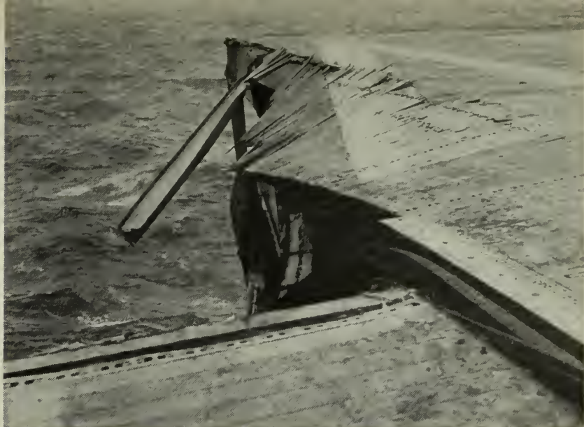
GREEN SEA broke over Valley's deck ripping loose an area 70 feet long from the carrier's port side.
